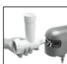
5. Turn the stand mixer attachment knob clockwise to secure grinder to mixer.
