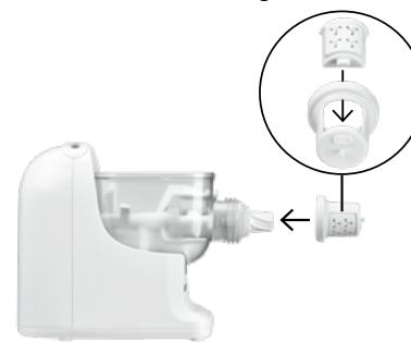
7. Use the locknut (5) to secure and lock the pasta disc holder (4) into place.
