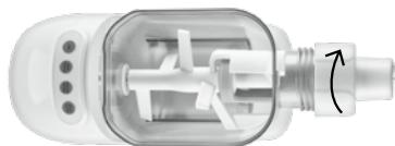
8. For extruding pasta, push the cutting tool (3) onto the disc holder (4) until secure. Position so the window of the cutting tool is framing the pasta disc.
